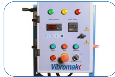
Electric Control Panel Elektrik Panosu
